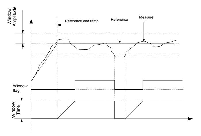
The parameters for the amplitude values for the relative windows and the minimum wait time are set using the modbus registers at addresses beginning with 35140.
