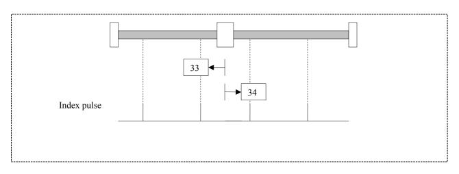
With the type 33 homing procedure, the initial direction is anti-clockwise; with type 34, it is clockwise. The reference (home) position is on the first index pulse (resolver zero) that is found in the selected direction.
