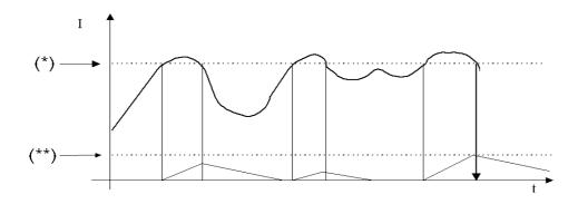
When the current exceeds the calculated maximum (\*\* the lesser value between parameters 111 and 112), the time on a timer is increased. When the current level then falls below the maximum level, the time on the timer is decreased. If the time on the timer exceeds a preset value (\*\* = parameter 32771), an error is signalled. This is a safety function provided to the user for protecting the application. The associated flag is C1D I ERROR.
