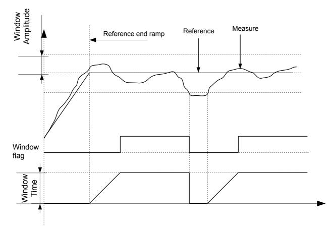
If the measured value of the specific measurement reaches the programmed reference value (at the end of the ramp, if applicable) and differs from the reference value by an amount that is less than the amplitude of the acceptance window (which can be set by the user), as indicated in the figure as *Window Amplitude*), the wait time is increased within the acceptance window.
