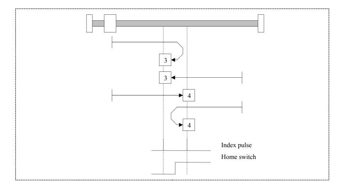
With types 3 and 4, the initial direction of movement depends on the state of the home switch. The reference (home) position is on the index pulse (resolver zero) to the left (type 4) or right (type 3) of the switching point of the home switch. If the starting position is such that a reversal of direction is required, the reversal takes place after the state of the home switch changes.
