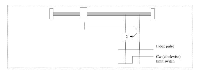
With this type of homing, the direction of initial movement is clockwise toward the clockwise limit switch, if it is inactive. The reference (home) position is on the first index pulse (resolver zero) to the left of the clockwise limit switch, when the value on the latter switches to low.
