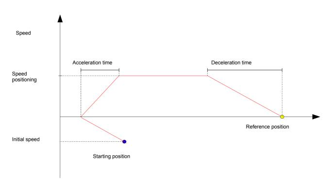
If there is insufficient space for stopping motion at the desired position, a profile of the following type is run:
