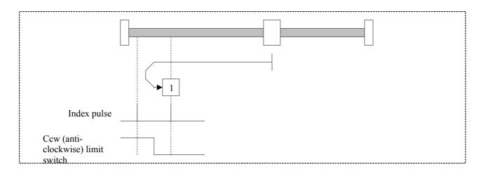
With this type of homing, the direction of initial movement is anti-clockwise toward the anti-clockwise limit switch, if it is inactive. The reference (home) position is on the first index pulse (resolver zero) to the right of the anti-clockwise limit switch, when the value on the latter switches to low.
